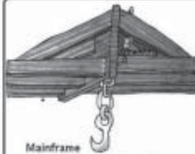
Mainframe Holds up the barn roof
